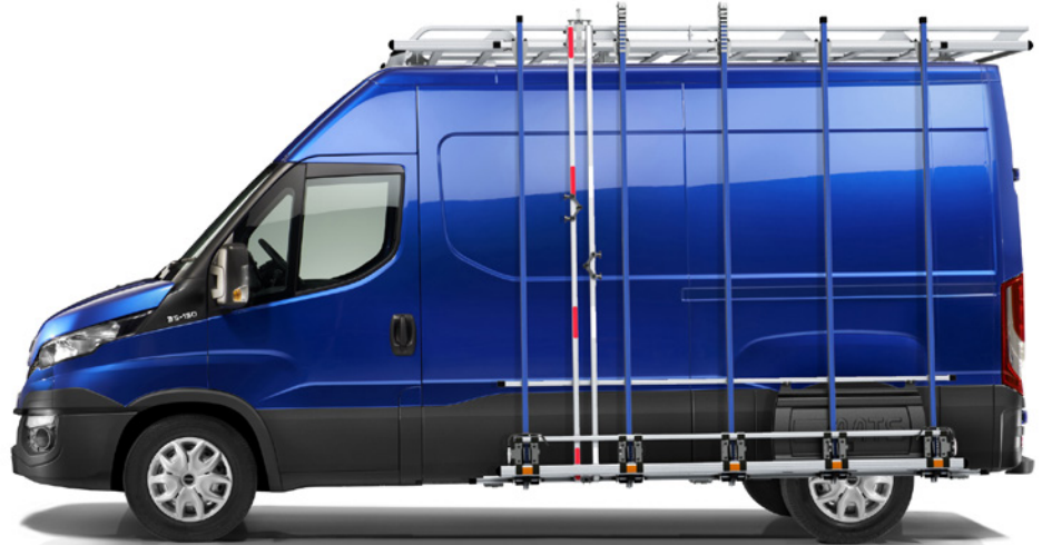
Superior, flush-folding system with multiple holes for attaching the securing poles
