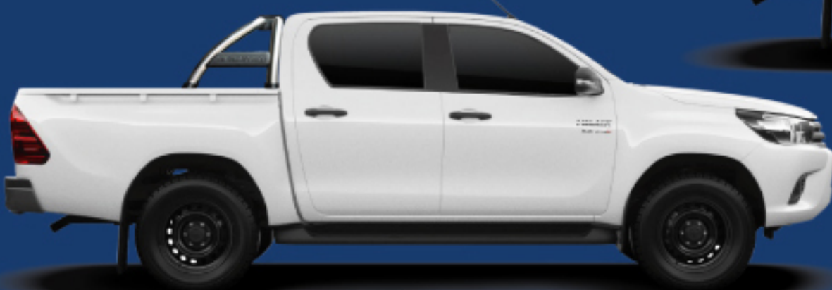
CB-766/CE-766 Stainless Steel Roll Bar Stainless steel tube \varnothing 3" (SUS201/TP304) with plastic injection cross bar with CARRYBOY logo.
