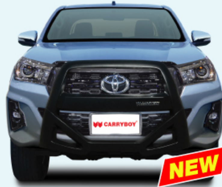
CB-771 Front Nudge Guard The FRP front nudge guard produced by RTM process, which give a strong, durable structure, and a 2 side smooth-finished surface. CB-771 comes in 3 different coloring styles, all mat black, two-tone, and color coated.
